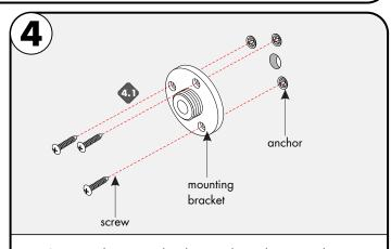
4.1 Secure each mounting bracket onto the anchors using the appropriate hardware.
