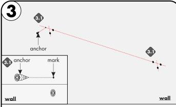
3.1 Align and then tap each anchor onto the marks until the threaded section. Followed by tightening the anchors with a Phillips screw driver. (Anchors not provided)
