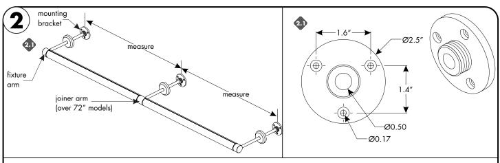
2.1 Measure the distance from one mounting bracket to the next. Then mark these location to the wall. Use the reference detail of mounting bracket above, for any additional information.
